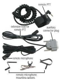
The TMAA10-04 remote PTT kit plugs into the radio's auxiliary connector. This kit uses the remote electret microphone to replace communication through the usual rugged microphone. The rugged microphone can still provide hookswitch operation, if this is required.
