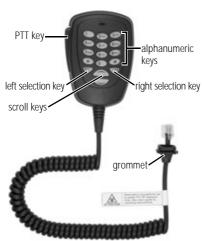
The TMAA02-08 keypad microphone plugs into the microphone socket on the graphical-display radio control head, and enables users to make calls to other radios, groups, or to a PABX or PSTN. The types of call that you can make depends on the way your radio has been programmed.
