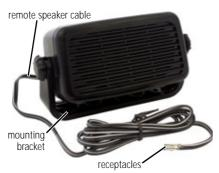
The TMAA10-03 remote speaker (for the 25W radio) and the TMAA10-06 remote speaker (for the 50W/40W radio) are installed in parallel with the radio's existing internal speaker. The remote speaker can then be installed at some distance from the radio, or it can be used to increase the volume of the audio from the radio's existing internal speaker.
